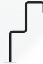
Edge backfilled with stainless steel. The edge backfilled with a steel profile or flat bar – it should be used in the zones with intensive traffic and high loads
