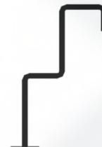
Edge backfilled with stainless steel. The edge backfilled with a steel profile or flat bar – it should be used in the zones with intensive traffic and high loads
