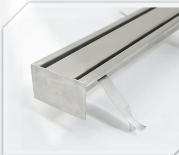
In our offer you can find **standard channels** made of **stainless AISI 304** or **acid-resisting AISI 316** steel. **Standard channels** are provided with bottom drop. In order to make assembly easier every channel is equipped with rectification screws and anchoring elements. They allow the **standard channels** to be leveled correctly and secured in concrete.
